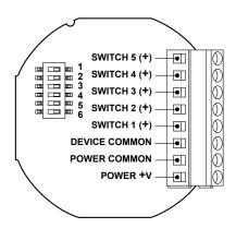
Connections: Field-wired through either of two 1/2-14 ports in housing.
